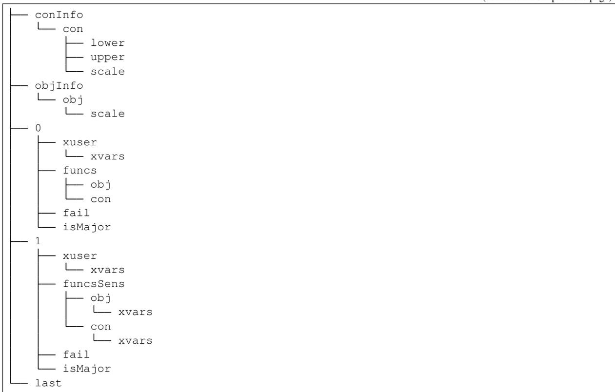
The main optimization history is indexed via call counters, in this example 0 and 1. Note that they do not match the major/minor iterations of a given optimizer, since gradient evaluations are stored separate from the function evaluation.
